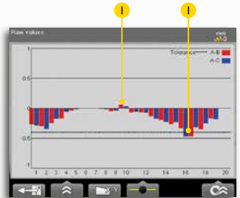
Taper values diagram. Taper out of tolerance (I).
